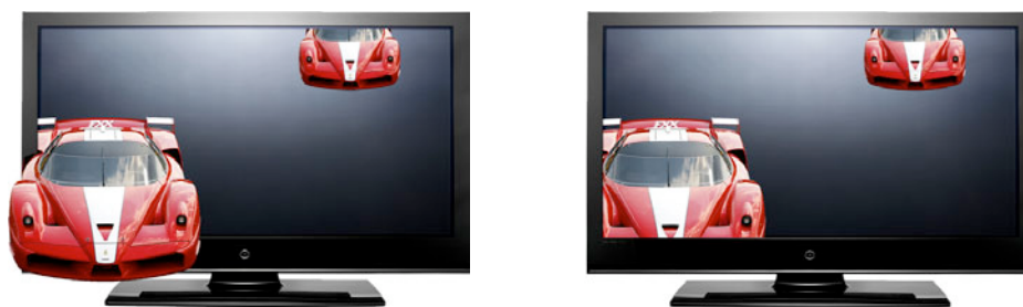
Figure 5: Frame violation (left: negative parallax, right: interposition)
